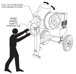
Figure 19. Mixing Drum Positioning
